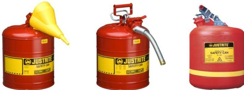
These are “Safety Cans” which are FM approved and/or UL Listed, and are required by OSHA when used by any business or commercial enterprise. Key required safety features include flame arresters, self-closing lids, pressure relief, and 100% leak testing. They generally range in purchase price from \$50 to \$150 and are available through industrial and safety supply distributors.
