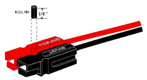
The contacts go in the housings in only one way. Insert the contacts with their sharp edge down against the flat spring that is in the housing. They should slide in and click. If you do not hear a
